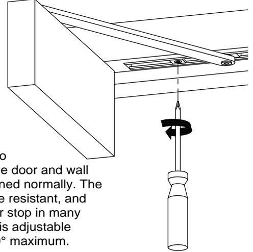
The deadstop helps to prevent damage to the door and wall when the door is opened normally. The deadstop is not abuse resistant, and cannot replace a door stop in many situations. Deadstop is adjustable between 80° and 120° maximum.
