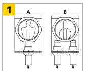
Select cam shape for keyswitches. Mortise cylinder and second switch sold separately.
